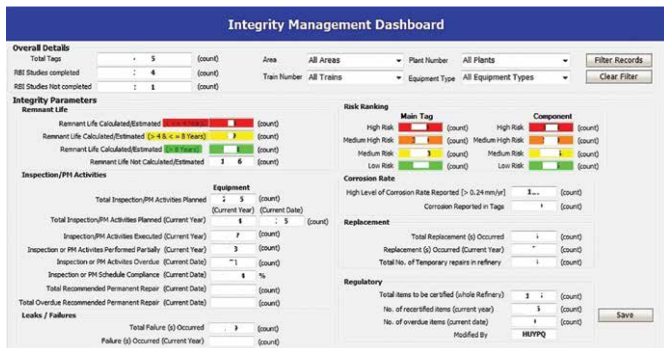
Figure 3. CIMS dashboard window.
